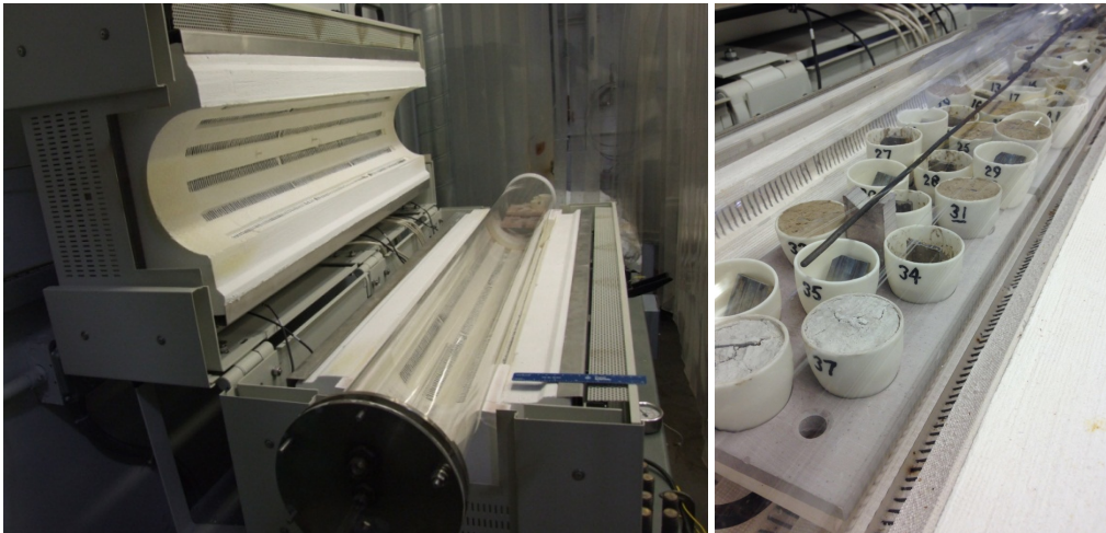
Figure 9 - Corrosion Test Set-Up
