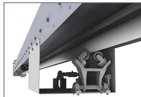
Lance tube / feed tube articulated center support
