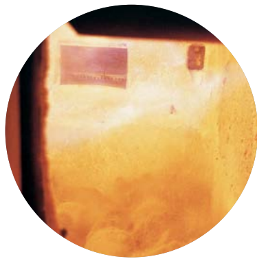
The thermal mass of the bubbling bed provides stability for fuel variations.
