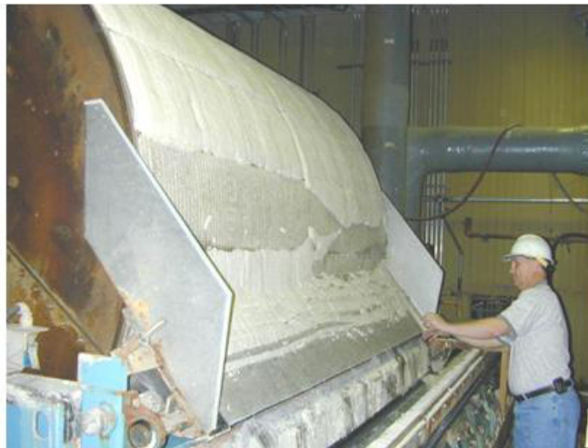
Figure 9 – Rotary drum filter
