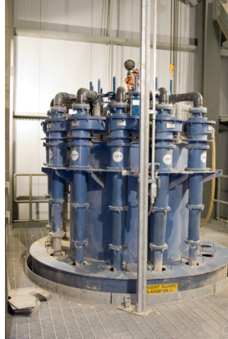
Figure 8 – Hydroclones require substantially less real estate compared to a thickener.
