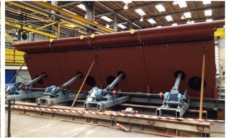
For small to medium power input, the grate has two boiler panels up to 6.4 m wide (left). For larger power input, the grate has four boiler panels up to 12.8 m wide (center and right).
